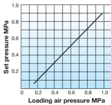
Basically, the set pressure to the loading air pressure is as shown on the left.
