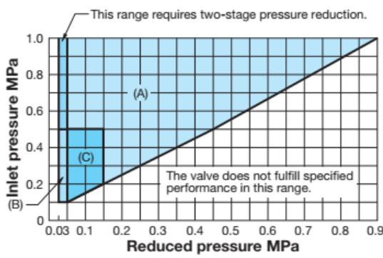
Find the intersection point of the inlet and reduced pressures. If the intersection point is within any of the ranges shown in the chart above, the pressures are controllable.
