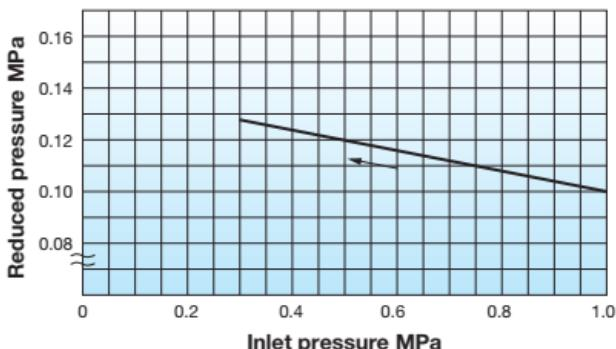
This chart shows variation in reduced pressure when the inlet pressure of 1.0 MPa is changed between 0.3 MPa and 1.0 MPa while the reduced pressure is set at 0.1 MPa.
